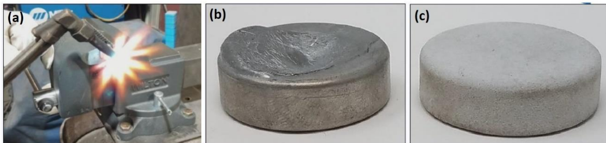
Figure 8 – Torch testing study: (a) torch exposure at cutting distance; (b) Uncoated Al 4032; (c) PEO-coated Al 4032.
